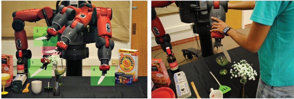
Fig. 1. Zero-G feedback: learning trajectory preferences from suboptimal zero-G feedback. (Left) Robot plans a bad trajectory (waypoints 1–2–4) with knife close to flower. As feedback, user corrects waypoint 2 and moves it to waypoint 3. (Right) User providing zero-G feedback on waypoint 2.
