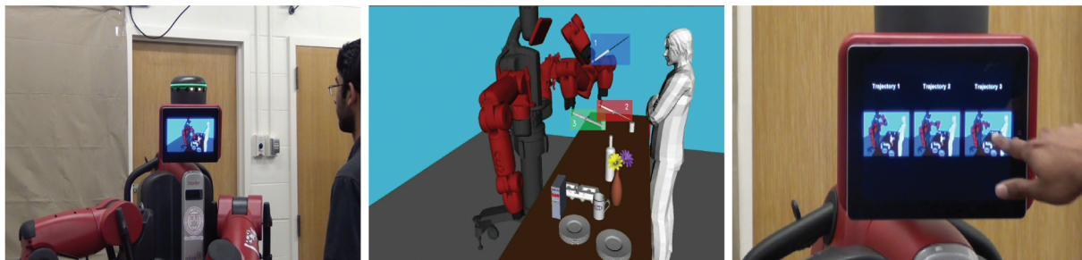
Fig. 2. Re-rank feedback mechanism. (Left) Robot ranks trajectories using the score function. (Middle) Top three trajectories on a touch screen device (iPad here). (Right) As feedback, the user improves the ranking by selecting the third trajectory.
