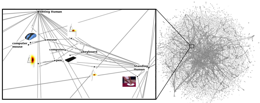
Figure 6.2: A visualization of the RoboBrain graph on Nov 2014, showing about 45K nodes and 100K directed edges. The left inset shows a zoomed-in view of a small region of the graph with rendered media. This illustrates the relations between multiple modalities namely images, heatmaps, words and human poses. For high-definition graph visualization, see: http://pr.cs.cornell.edu/robobrain/graph.pdf
