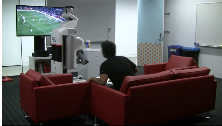
Figure 3.15: Robotic experiment: A screen-shot of our algorithm running on PR2. Without learning robot blocks the view of the human watching football. http://planit.cs.cornell.edu/video
