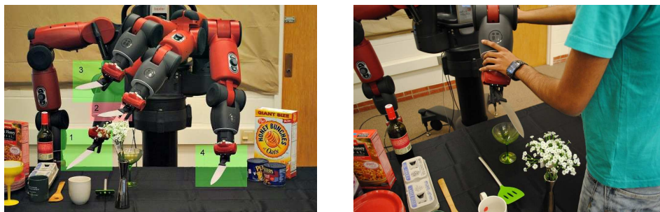
Figure 2.3: Zero-G feedback: Learning trajectory preferences from sub-optimal zero-G feedback. (Left) Robot plans a bad trajectory (waypoints 1-2-4) with knife close to flower. As feedback, user corrects waypoint 2 and moves it to waypoint 3. (Right) User providing zero-G feedback on waypoint 2.
